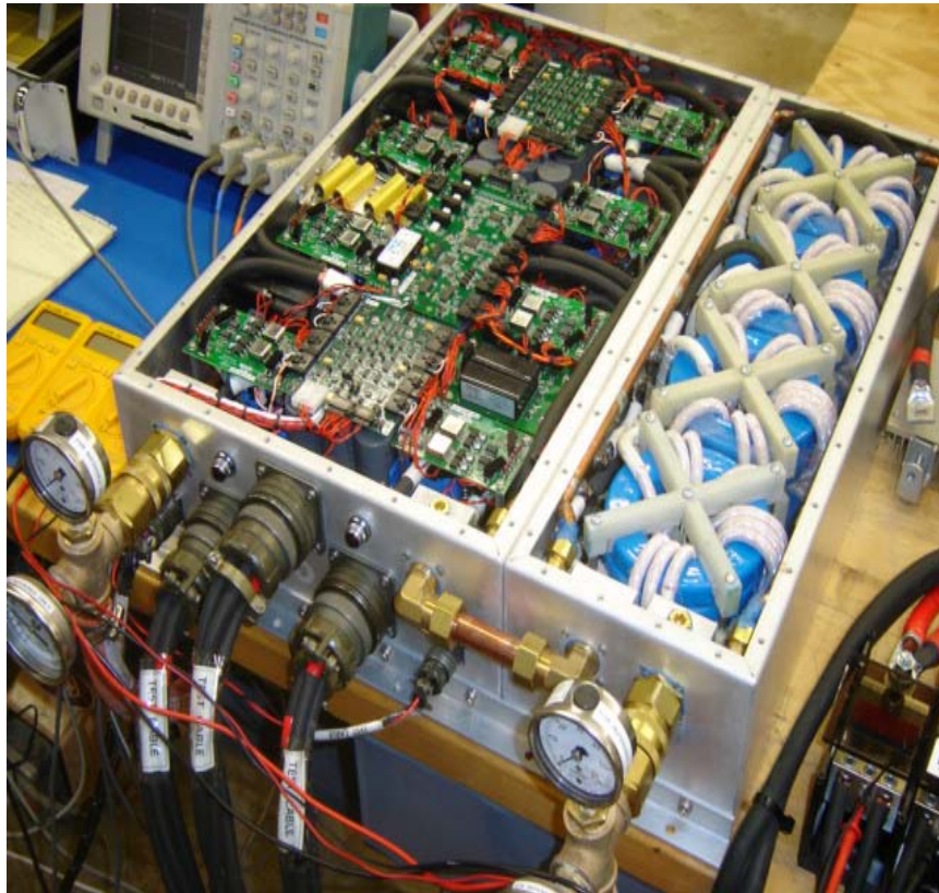
150kW Hybrid Vehicle Bi-Directional DC/DC Converter
